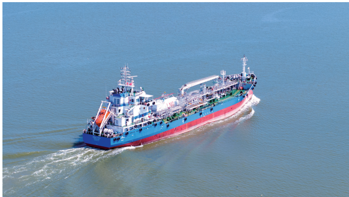
江门造新型绿色低碳双燃料加油船“AMALTHEA”轮。 This is AMALTHEA, a new low-carbon dual-fuel refueling vessel manufactured in Jiangmen.
